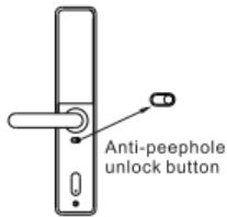
Turn the button to enable and disable the function and prevent kids or pet unlock the door by accident.
